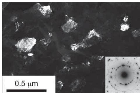
Figure 4. Structure of Mo after deformation to three revolutions ( $e = 6.5$ ) at 290 K. Dark-field image in reflection (110) and electron diffraction patterns.
