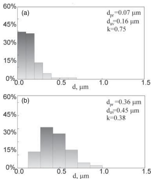
Figure 7. Size distribution diagrams of structural elements: (a) after deformation ( $e = 6.5$ ) and (b) after subsequent irradiation mode 4.
