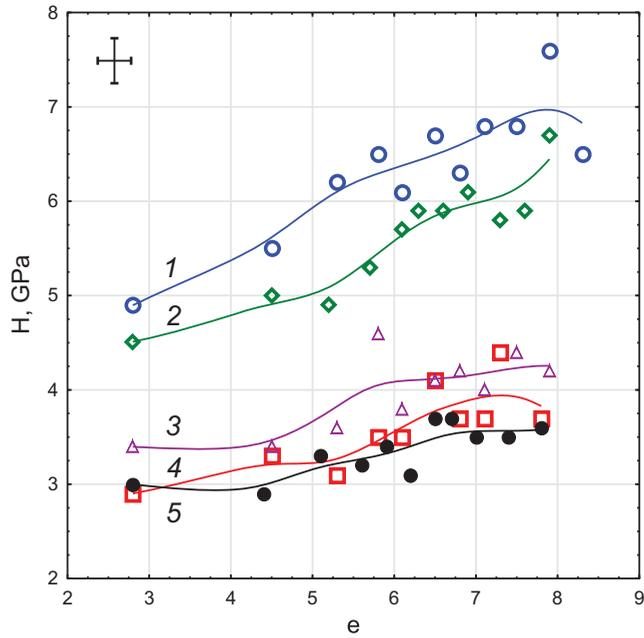
Figure 5. Microhardness of Mo after various modes of processing (deformation plus subsequent irradiation with  $\text{Ar}^+$  ions with energies of 20 keV): (1) after deformation at 290 K; (2) mode 1; (3) mode 2; (4) mode 3 and (5) mode 4.
