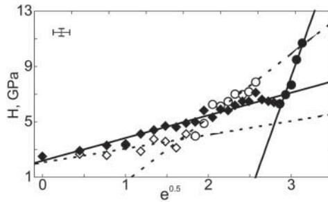
Figure 3. Microhardness of Mo deformed at two different temperatures as a function of  $e^{0.5}$ : (◆) first stage, 290 K; (●) second stage, 290 K; (◇) first stage, 80 K and (○) second stage, 80 K.
