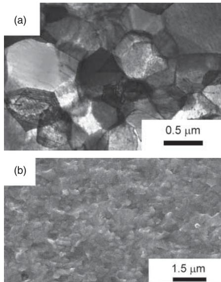
Figure 6. Structure of Mo after the optimal mode of deformation ( $e = 6.5$  at 290 K) and irradiation (mode 4):  $d_{av} = 0.45 \mu\text{m}$ ; (a) TEM and (b) SEM.
