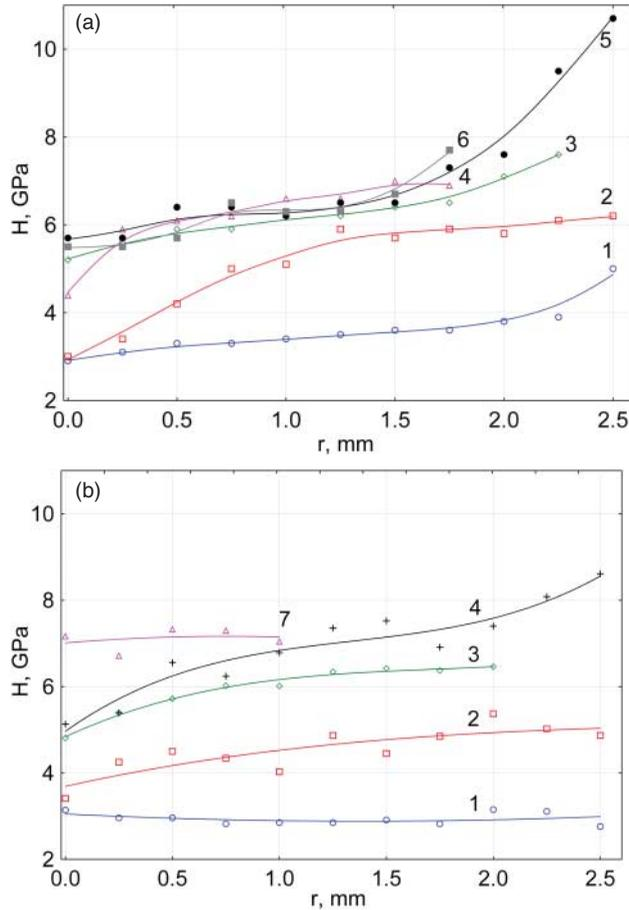
Figure 1. Microhardness of Mo vs. sample radius: (a) 290 and (b) 80 K. Rotation angle of the anvil: (1) 15°, (2) 180°, (3) 1 rev., (4) 3 rev., (5) 5 rev., (6) 10 rev, and (7) 1.5 rev.
