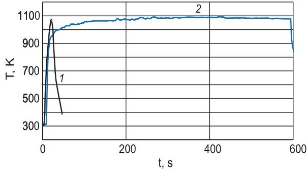
Figure 2. Temperature–time curves of Mo-deformed samples irradiated with  $\text{Ar}^+$  ions: (1)  $j = 400 \mu\text{A cm}^{-2}$  without holding and (2)  $j = 300 \mu\text{A cm}^{-2}$  with holding.
